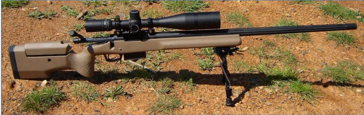
Figure 2. Custom .308Win APRS-LR Long Range rifle tested by the Author. 0.3MOA groups were the norm.
