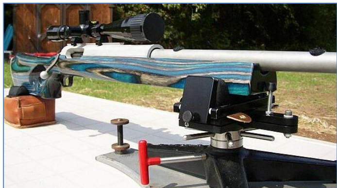
Figure 1. American custom built Benchrest rifle in 6mmBR capable of shooting 5-7" groups at 1000 yards.
